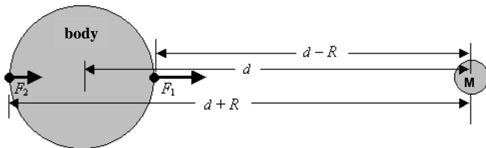
$$F_2 = \frac{GMm}{(d + R)^2} \quad F_1 = \frac{GMm}{(d - R)^2} \quad \Delta F = F_2 - F_1 = \frac{GMm}{d^2} \left[ \left(1 + \frac{R}{d}\right)^{-2} - \left(1 - \frac{R}{d}\right)^{-2} \right]$$
