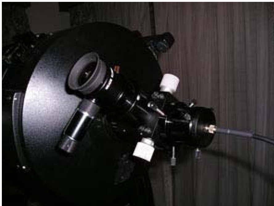
Figure 12 The flip mirror, the reticle eyepiece and the fiber optic cable
