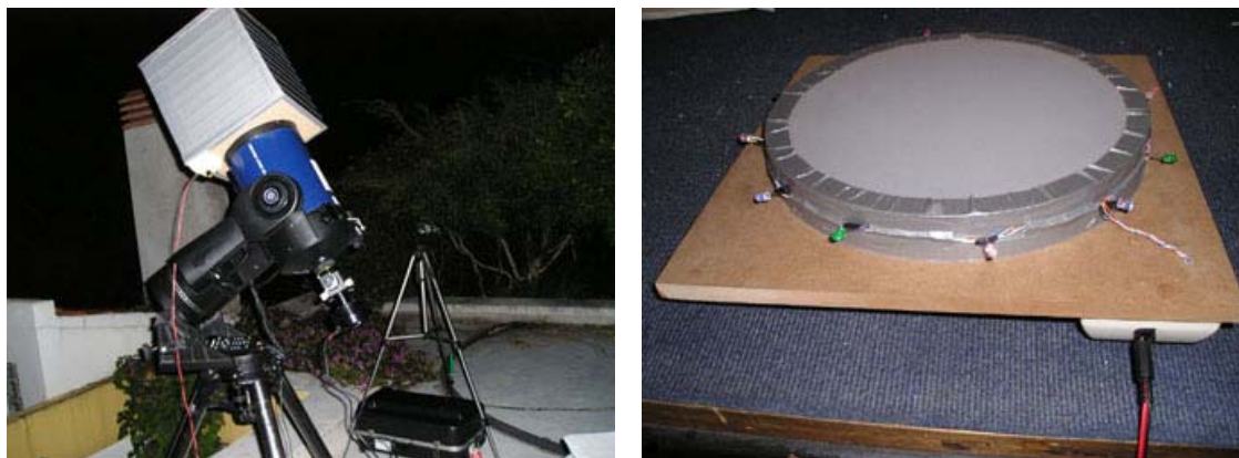
Figure 13 The constructed lightbox at field, and a detail showing its translucent layer that results evenly illuminated by twelve colour LEDs, strategically placed under it
