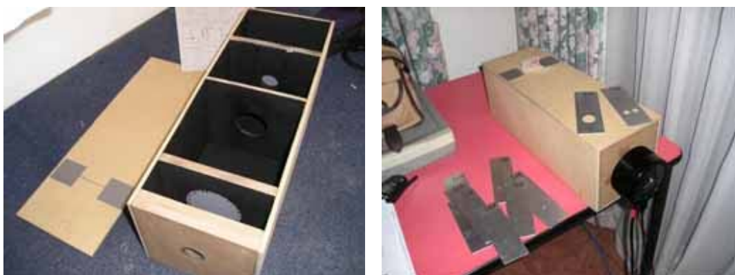
Figure 16 The low-level light source has a LED that brights at a very stable level; the amount of light reaching the CCD is adjusted by introducing different calibrated holes
